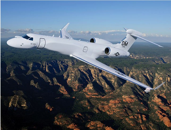
Figure 10: Illustration of an EA-37B Compass Call . The aircraft's stats sheet describes the EA-37B as an electromagnetic attack aircraft that “denies, degrades and disrupts adversary command, control, communications, radars, and navigation systems to restrict enemy electromagnetic-based battlespace coordination. The weapon system neutralizes enemy air defenses by preventing the transmission of essential information between sensors, weapon systems and control networks.”
