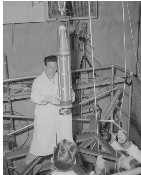
Figure 1: The first United States satellite, Explorer 1, being mated to the launch vehicle in 1958.
