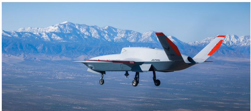
Figure 1: The XQ-67A Off Board Sensing Station is a second-generation autonomous collaborative air platform.
