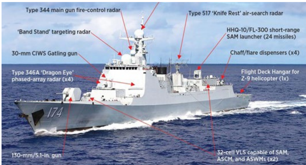
Figure 2: Type 052D Luyang III class destroyer. The PLAN's primary AAW sensor is the Type 346 radar—known to NATO as the Dragon Eye—which is installed on its Type 052C Luyang II-class destroyers. These destroyers are also armed with long-range HHQ-9 SAMs that are variants of the Russian Almaz-Antey S-300. A larger, follow-on Type 052D Luyang III-class of destroyers have upgraded Type 346A Dragon Eye radars and are equipped with 64 rather than 48 VLS tubes.
