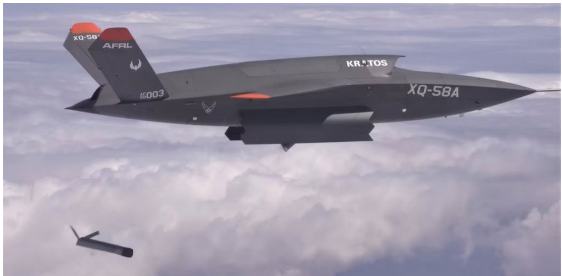
The XQ-58 Valkyrie is an uncrewed aircraft that the U.S. Air Force is flying at Eglin AFB to develop and test autonomy software. Source: Air Force Research Laboratory Photo
