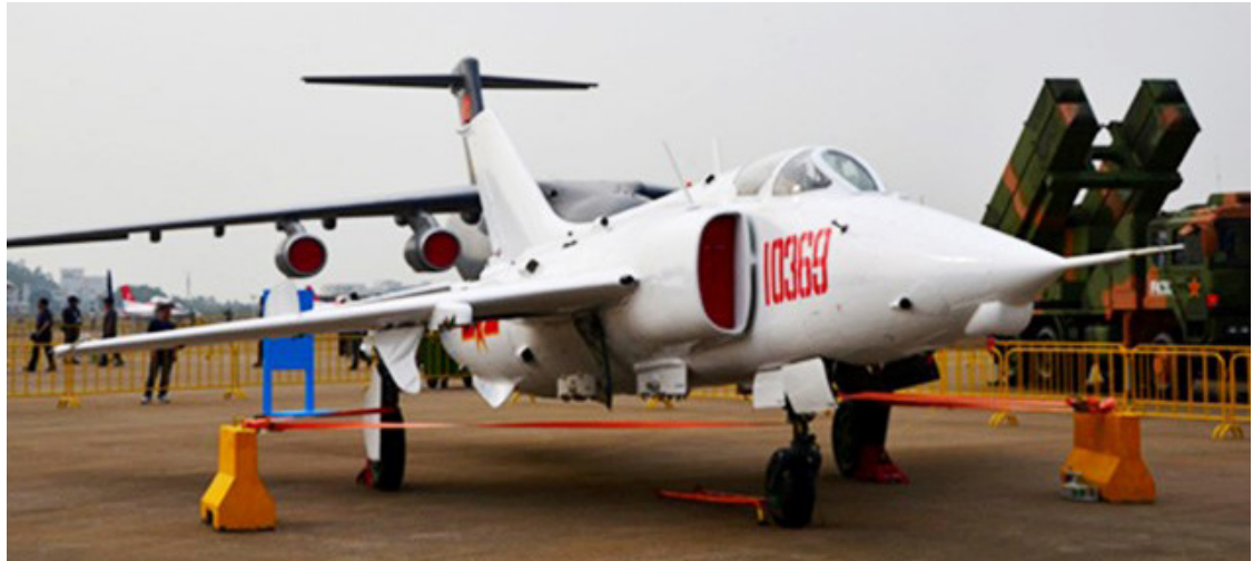
Image: A Q-5 airframe converted into a UCAV Source: Photo courtesy of Mike Dahm from his personal collection.
