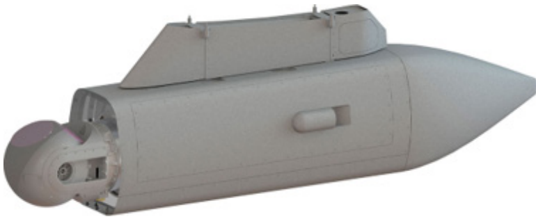
Figure 11: Airborne Laser Communications System payload. High-altitude C2ISR platforms that operate above usual weather phenomena offer good initial candidates for integration of such airborne optical terminals.
