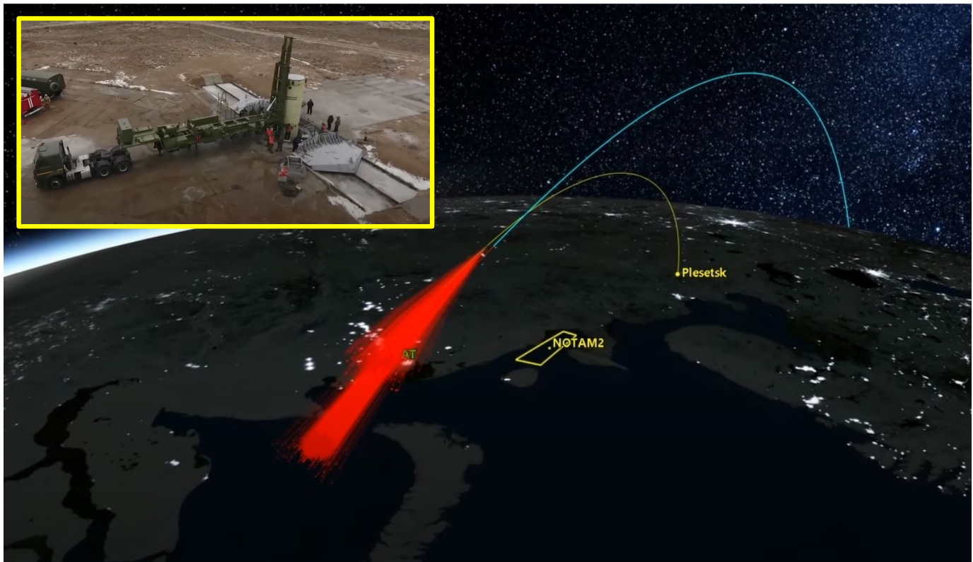
Figure 6: Physics-based recreation of November 15, 2021 Russian ASAT test that shot down the Russian satellite Cosmos 1408 (orbit shown in blue) using a direct-ascent kinetic weapon (trajectory shown in yellow), creating the resulting debris field (hypothetical depiction in red). Overlay is of the A-235 Russian ASAT system believed to have been used in the test. Image source: AGI
