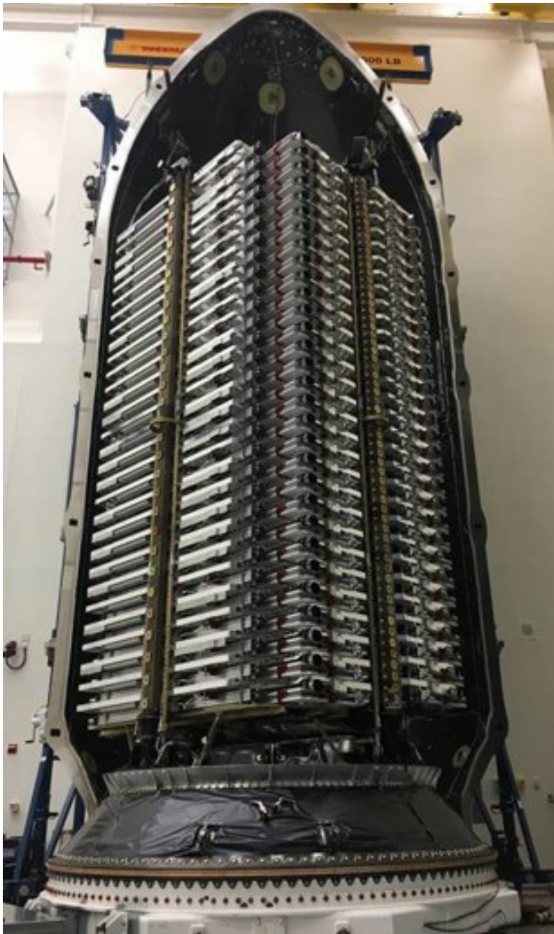
Figure 13: 60 SpaceX Starlink satellites stacked into Falcon 9 launch vehicle fairing prior to launch. Establishing and maintaining proliferated constellations will require satellites to be manufactured at an unprecedented rate for the space industry.
