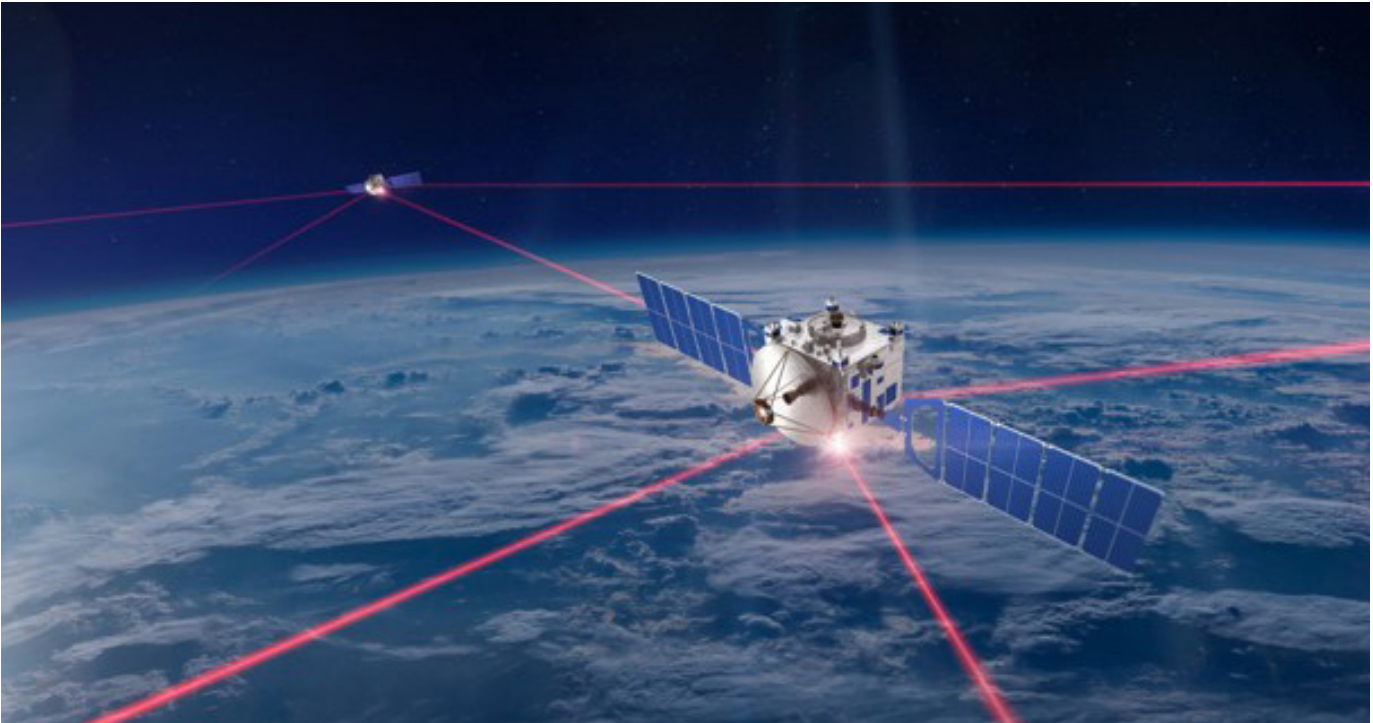
Figure 10: Artist depiction of a segment of a LEO constellation supported by laser communications. Equipping each satellite with multiple optical communications terminals forms a “mesh” network that provides numerous diversified connectivity paths through which to route data and information through space.
