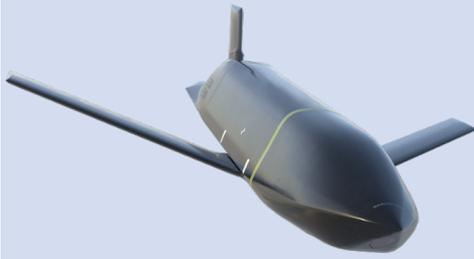
JASSM and LRASM are low observable, highly survivable munitions equipped with GPS-aided INS for guidance, imaging infrared seekers, and a pattern-matching autonomous target recognition capability designed to strike high-value, heavily defended fixed and relocatable targets. One of the principal authors of the 2018 NDS identified JASSMs and LRASMs as examples of munitions that "are must-buys to increase the defensibility of Taiwan and the Baltics." (see endnote 50).
