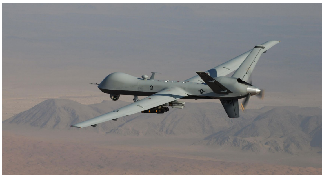
Figure 3: MQ-9 Reaper, armed with GBU-12 Paveway II laser guided munitions and AGM-114 Hellfire missiles
