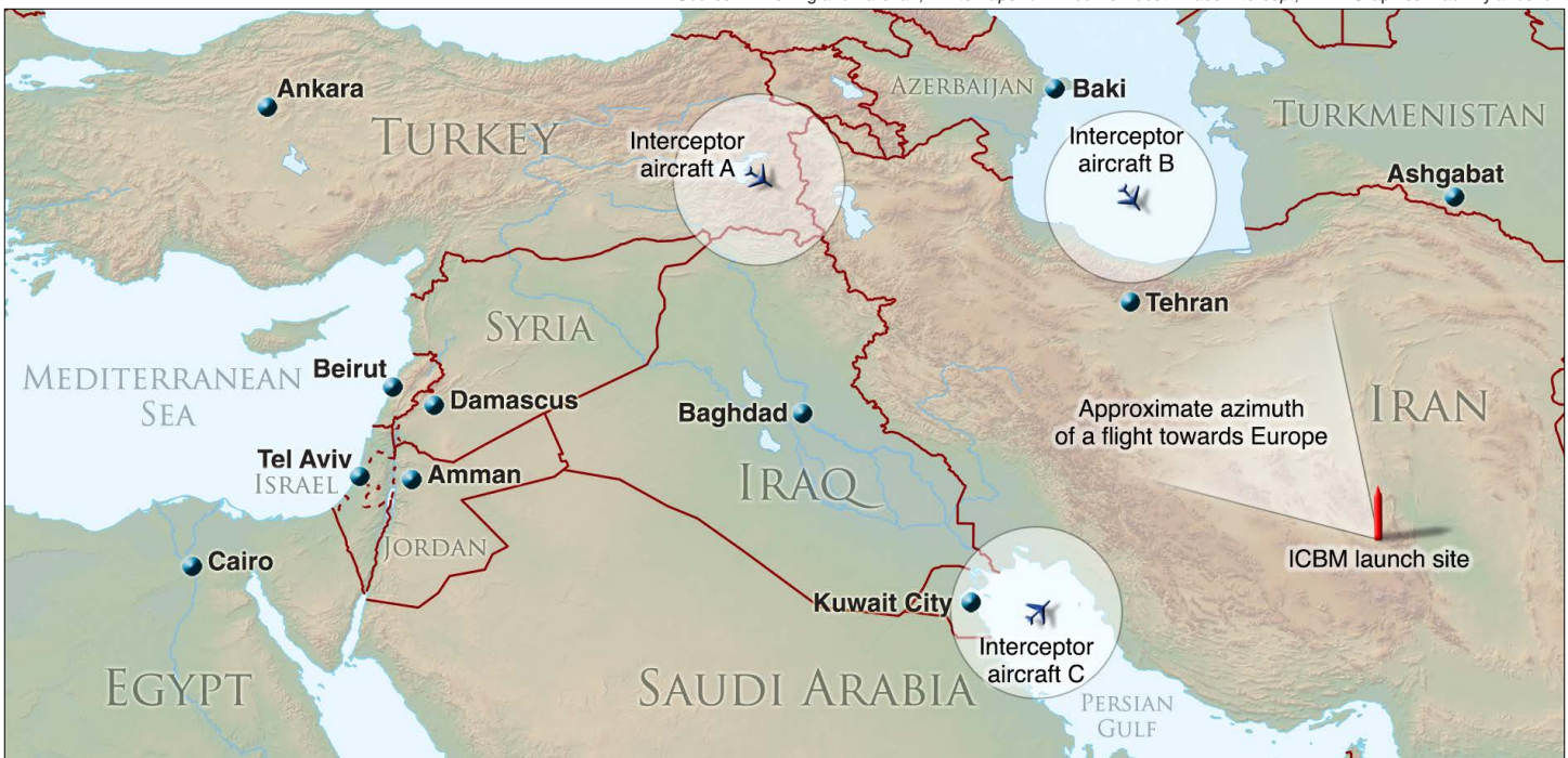
Figure 2: This figure depicts the patrol and launch orbits of a 350-kg (770-lb) multi-stage airborne boost phase interceptor with a 3km/second divert performance capability against known ballistic missile designs (divert performance refers to the energy margin available to an interceptor to remove internal guidance and targeting aim error). The notional launch site of an Iranian missile is depicted by the red missile, with an azimuth fan aimed at targets in Europe.
