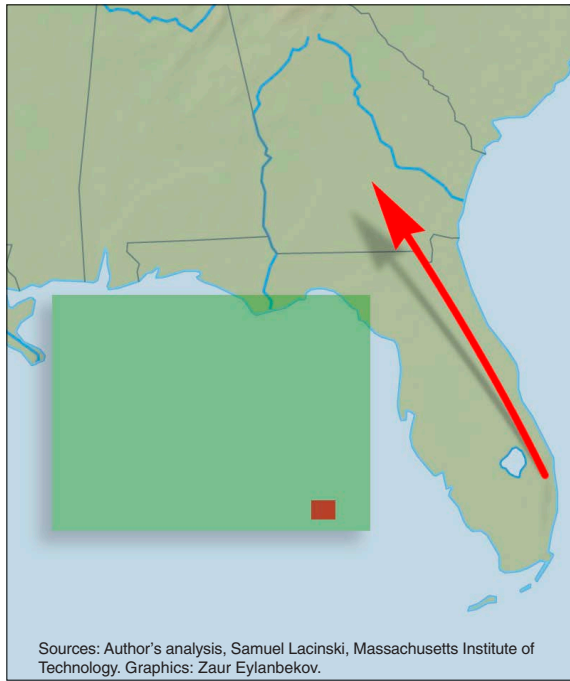
Figure 3: The green rectangle in this figure depicts the approximate launch envelope of a 700-kg (1,500-lb) two-stage airborne boost phase interceptor targeting a multi-stage liquid propelled ICBM with a 10,000-mile range. This green launch zone is outside of the territorial overflight of the “adversary country,” which in this case is represented by Florida (excluding the panhandle) and is outside all but the most advanced surface to air missile ranges. The single small red square in the bottom right corner represents the only area in the space where a boost phase interceptor could not fully satisfy all intercept criteria.
