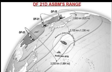
Possible layered ASBM strike architecture, with 1,000, 2,000, and 3,000 km range ASBM strike assets. The DF-25 designation is only a notional representation of a follow-on 3000-kilometer range ASBM capability
