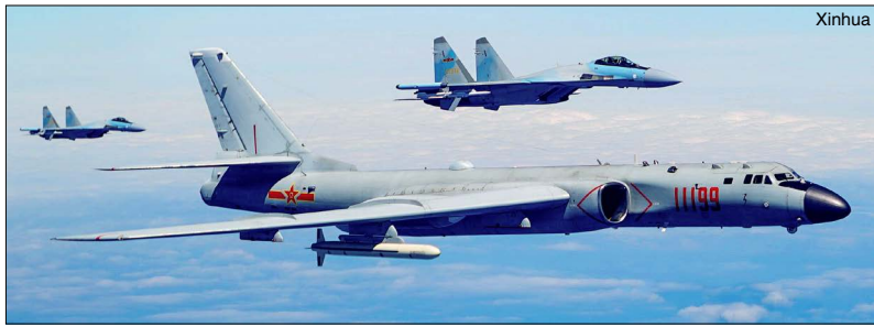
Above: A Chinese H-6K bomber (variant of the Russian Tu-16) conducting patrols near Taiwan with Su-35 escort fighters. H-6 variants have been equipped with modernized air-launched anti-ship weapons, such as the YJ-81 and YJ-83.
